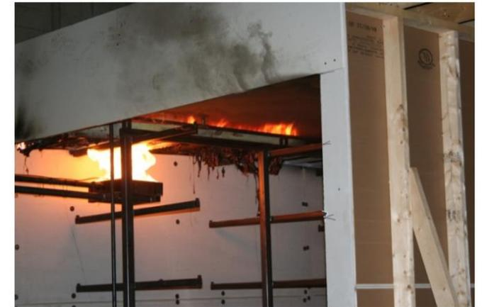
NUREG/CR-7010, Vol. 2: Cable Heat Release, Ignition, and Spread in Tray Installations During Fire (CHRISTIFIRE) Phase 2: Vertical Shafts and Corridors
